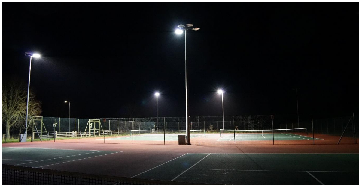
Existing lighting - showing glare, light trespass and cool white lighting
