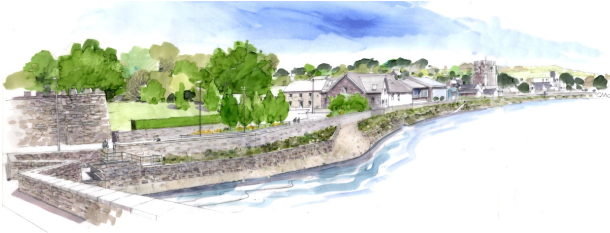
Plate 3-1: Illustration showing the proposed engineered riverbank with intertidal habitat development, with the flood wall visible along the crest.
