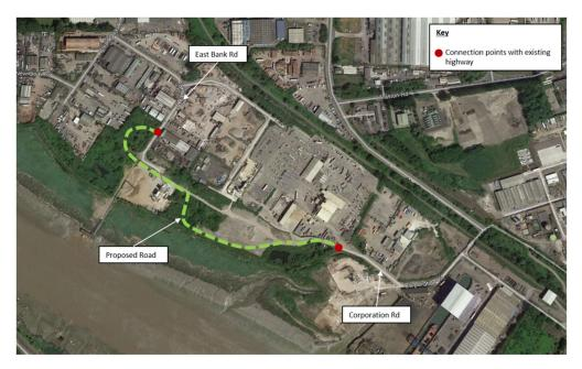
Figure 10 Proposed road showing connection points with existing highway (red dots)
