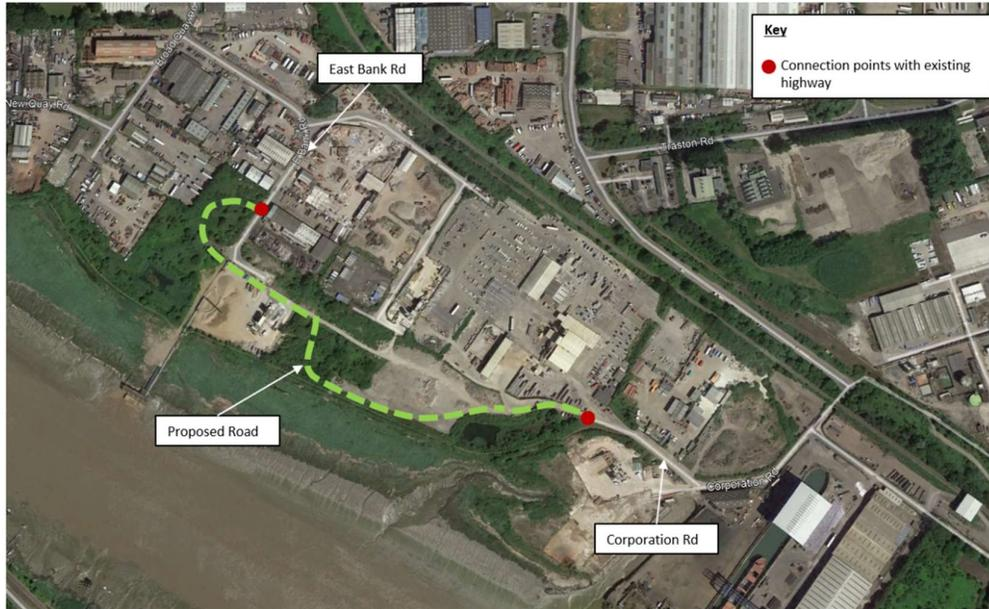
Figure 10 Proposed road showing connection points with existing highway (red dots)
